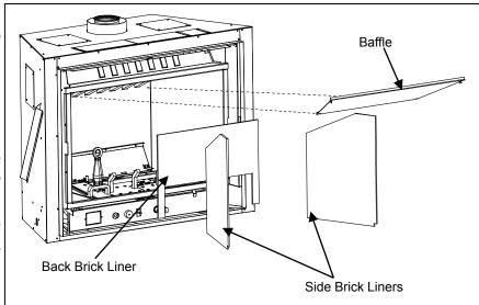
Figure 38: Cast Iron Brick Liner Installation.
